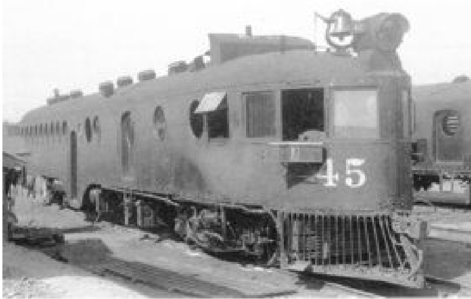
Appendix A, Top: Example of a McKeen car, showing pointed nose and round windows. Appendix B, Bottom: Side view of another McKeen car. Note flywheel on front set of wheels.
